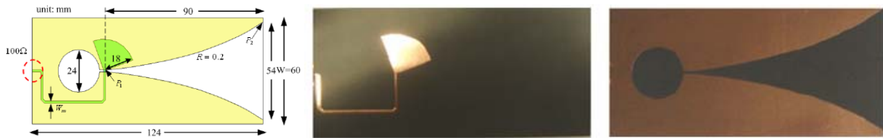
Fig. 10. 2-4GHz Vivaldi Antenna for through wall applications [22]
